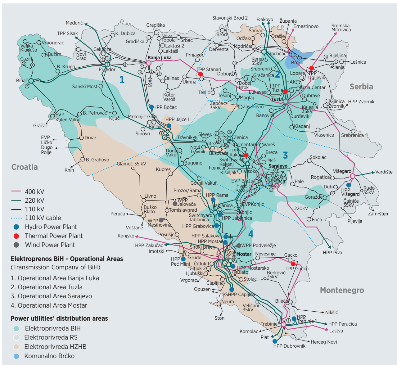
Figure 6 Map of the electric power system of BiH with operational areas of the transmission level (Elektroprenos BiH) and distribution areas of the public electric utilities, 31 December 2020, and power plants
